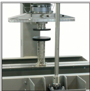
300kN UNIFLEX frame (50-C1601/FR) fitted with accessory for compression tests (50-C1601/4 and 50-C1601/KIT)
