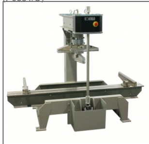
300kN UNIFLEX frame (50-C1601/FR) fitted with accessories for flags testing (50-C1601/2 and 50-C1601/KIT)
