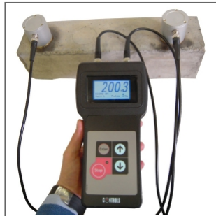
58-E4800 in use. Although the direction in which the maximum Energy is transmitted at right angle to the face of transmitting transducer, it is possible to detect pulses which have travelled through concrete in other directions: adjacent faces (semi-direct transmission) or same face (indirect or surface transmission).
