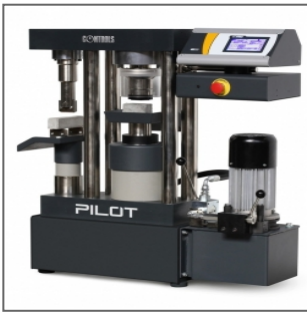
Double chamber 300/15 kN Pilot compression machine 65-L27C12 with incorporated compression and flexural jigs
