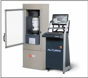
50-C20E82 AUTOMAX E-Modulus controlling a EN compression frame with three electronic compressometer-extensometer fitted to a cylindrical specimen
