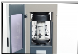
AUTOMAX E-Modulus. Determination of modulus of elasticity
