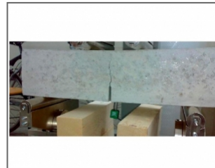
Concrete beam subjected to flexure loading with measurement of crack opening
