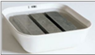
Plastic pan for water curing of three 40 x 40 x 160 mm cement prisms
